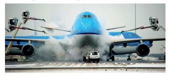
De-icing is performed with a liquid formed from at least 50% glycol, which is highly flammable, plus water.
