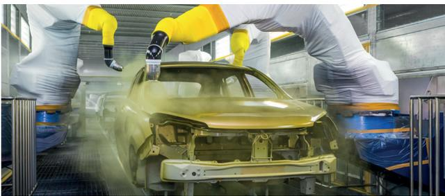
When atomised in the spray nozzle, mists can produce ignitable mixtures.
