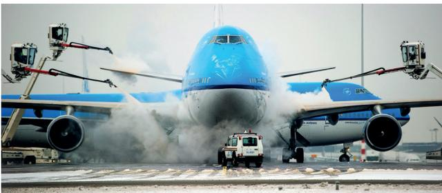
De-icing is performed with a liquid formed from at least 50% glycol, which is highly flammable, plus water.
