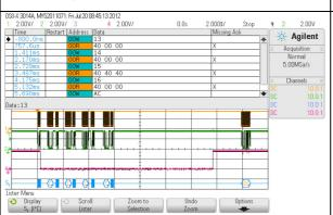
On the left side are 4 read cycles on the memory visible before the request 0xAC command occurs. In the memory cells 0x13 ... 0x16 is the scaling of the pressure output stored.
