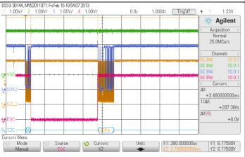
The handshake-solution, done by the additional EOC wire, is very elegant and is suitable to save time and power. The Master controller can be in sleep mode and will be awoken by an external interrupt on the positive slope of the EOC pin. Polling the level of the EOC wire is also possible.
