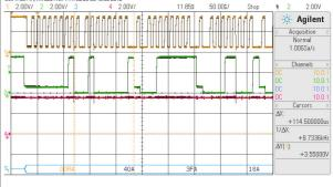
More detailed view of the readout frame: EOC is back to 3.6V. The slave ACK occurs as normal immediately after the neg. edge of the 8th clock impulse. The ACK from the master occurs with a little delay but this is allowed because the master generates the 9th clock impulse by itself at the right time.
