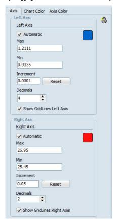
This functionality makes it possible to zoom in or out and change the scaling of the axis. To make manual changes the check box have to be deactivated and the entering of a new figure be confirmed with the Enter key (not by just clicking to the next box).
