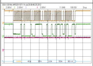
No acknowledge (NACK) from the master after reading out the 5<sup>th</sup> data byte. The "Missing Ack" that is recorded in the tables is not a mistake, it's a must.
