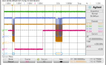
The simplest way to "detect" the end of a conversion (EOC) is to wait until the new data is definitely ready to read out. Being on the safe side; the conversion and the conditioning of the pressure and temperature value is completed after 8ms.
