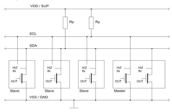
Pull-up resistors are needed at SDA and SCL. 1..10kOhm are recommended. In order to optimise the data rate or low power consumption, other resistance values are possible.
