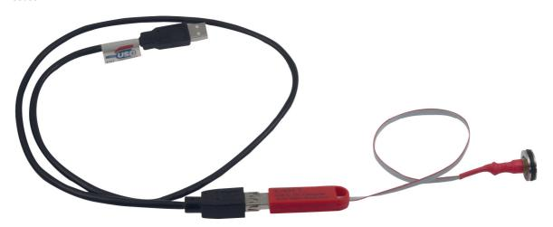
The K-404 converter is short circuit protected. The EOC-Pin is not connected and SDA and SCL are pulled up to the 3,3V supply by internal resistors. Please be careful by connection an oscilloscope with relation to earth because there is no galvanic isolation built in the converter.
