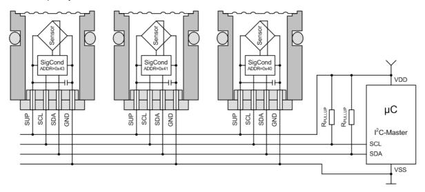
The bus capability is given by the physical (electrical) and the data link (protocol) bus layer.
