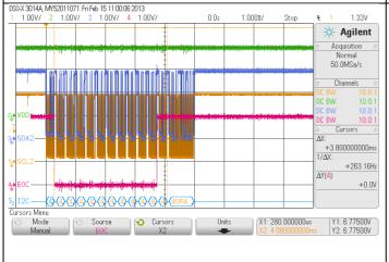
To save time without the additional EOC wire is possible by reading out the status of the pressure transmitter. There is no request needed, just a simple readout command for the first byte that contains the "Busy?" flag.
