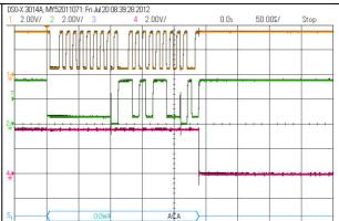
Nice to see: The ACK from the slave follows immediately to the negative edge of the 8th clock impulse (two times visible).
