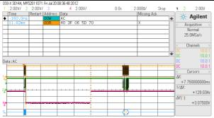
The EOC line is low for 7.75ms. The newest datasheet guarantees a conversion time below 8ms, typ. 6ms. To reach sample rates over 100 SPS it is a must to work with a high bit rate and to check the EOC line or to poll the STATUS byte.
