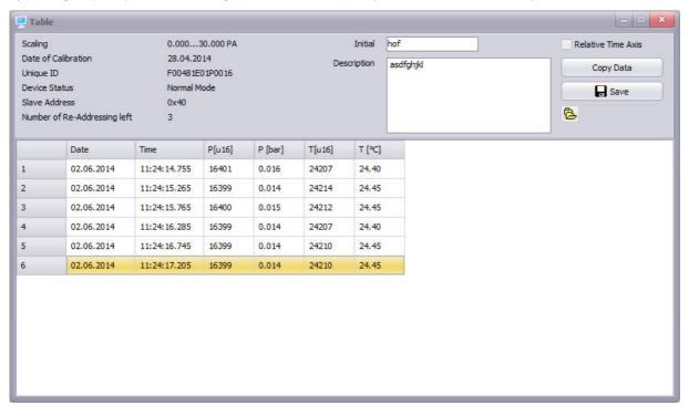
The table shows the data stored in the background of the monitor chart. Choose "Relative" or "Absolute Time Axis" before starting the data acquisition.
